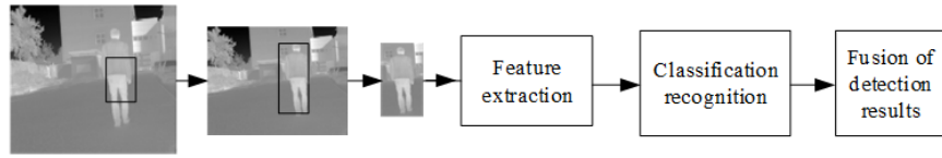
Fig. 6. Flowchart of multi-scale sliding window detection
