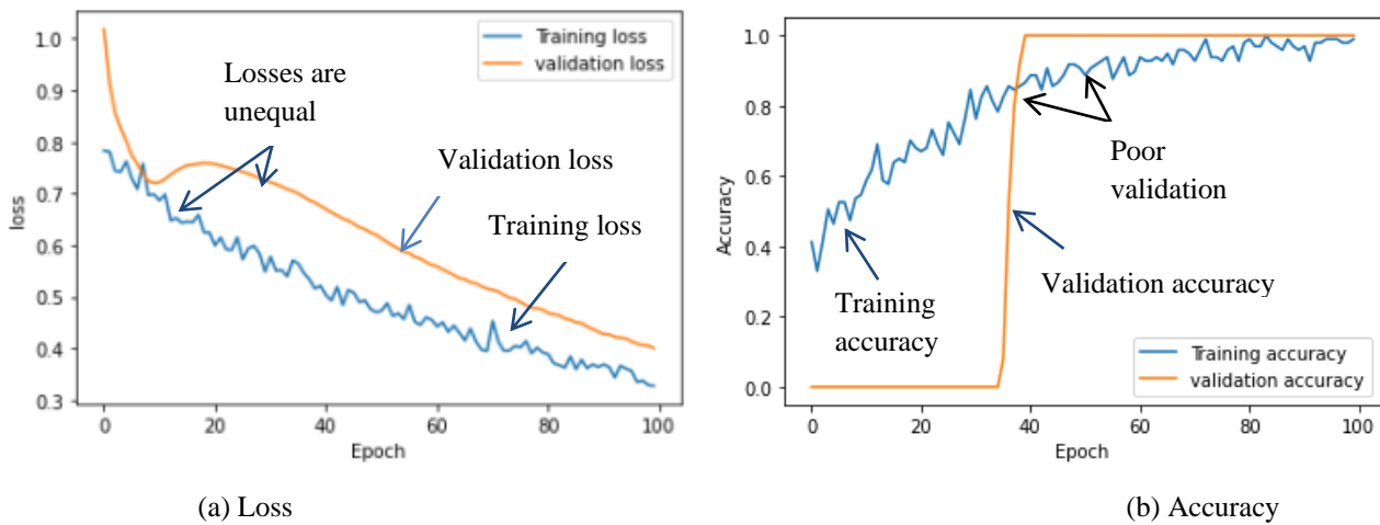
Fig. 4: Under-fitting model for epoch=100 for dataset L1(a)Loss and (b)Accuracy curves.
