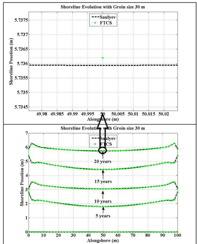
Fig. 25. Shoreline evolution in 20 years when T-head Groin size 30 m.
