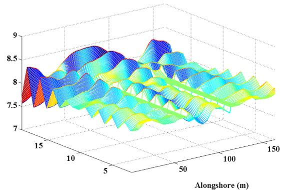
Fig. 12. Wave crest impact in 13 years when T-head groin 22 m.
