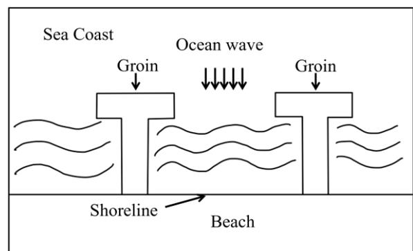
Fig. 3. Initial shoreline with configuration T-head groins.
