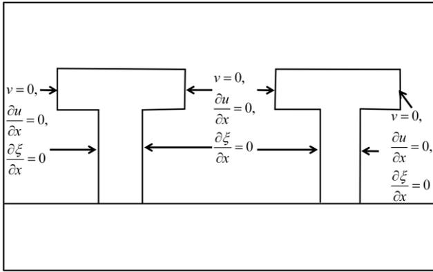
Fig. 6. Initial and boundary condition for T-head grain structure (1).
