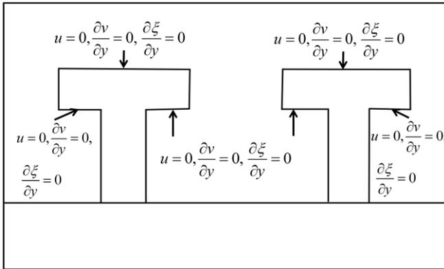
Fig. 7. Initial and boundary condition for T-head grain structure (2).
