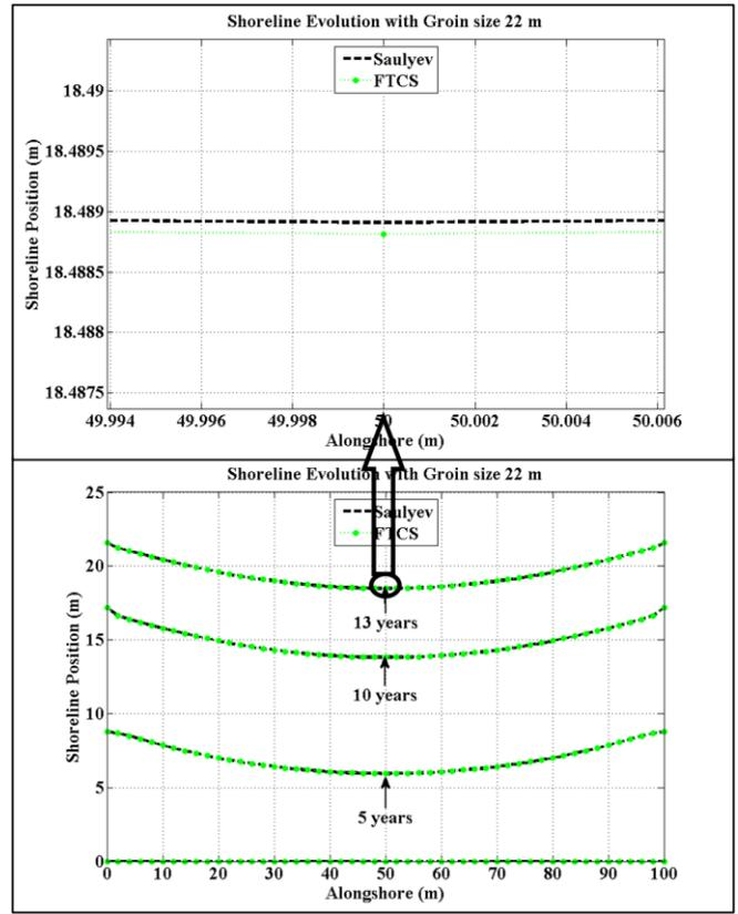
Fig. 21. Shoreline evolution in 13 years when T-head Groin size 22 m.
