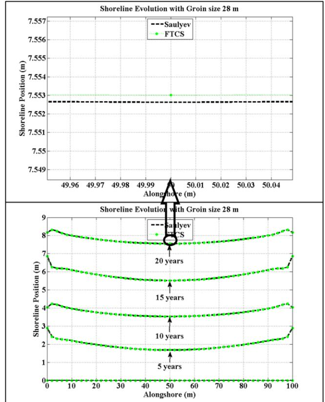
Fig. 24. Shoreline evolution in 20 years when T-head Groin size 28 m.
