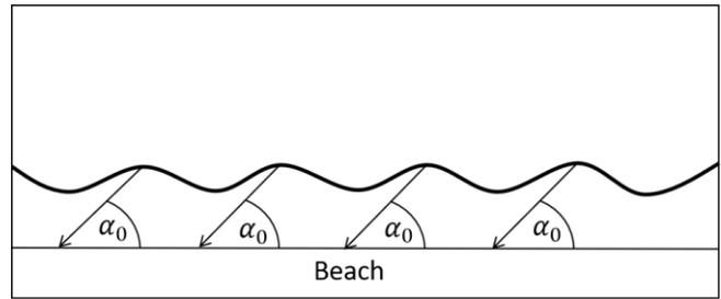
Fig. 1 Breaking wave crests impact angle when the beach is parallel to the  $x$ -axis
