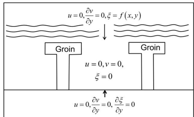
Fig. 5. Initial and boundary condition.
