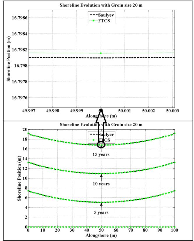
Fig. 20. Shoreline evolution in 15 years when T-head Groin size 20 m.
