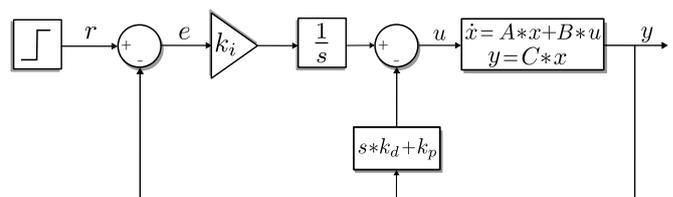
Fig. 5. I+PD controller block diagrams
