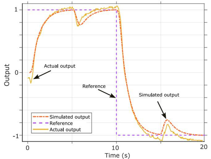
Fig. 10. Detailed view of the first output of the twin rotor MIMO system
