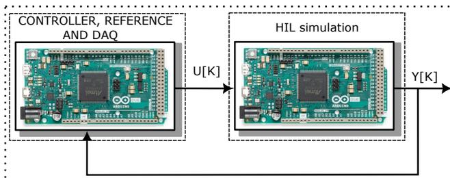
Fig. 3. Real-time simulation and control
