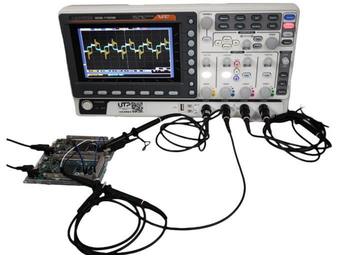
Fig. 15. HIL interconnection structure by using two Arduinos DUE
