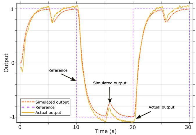
Fig. 9. First output of the twin rotor MIMO system
