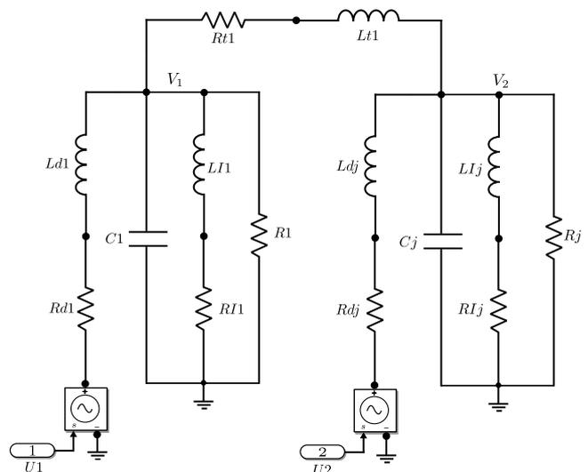
Fig. 7. Microgrid dynamic system.
