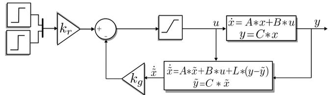
Fig. 6. Block diagram of Twin Rotor system
