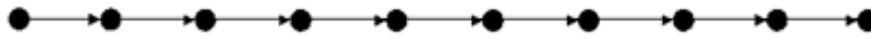
Fig. 2. Chain network containing 10 neurons. In this network, neuron i ( i > 1 ) receives only the signal from neuron i - 1 .
