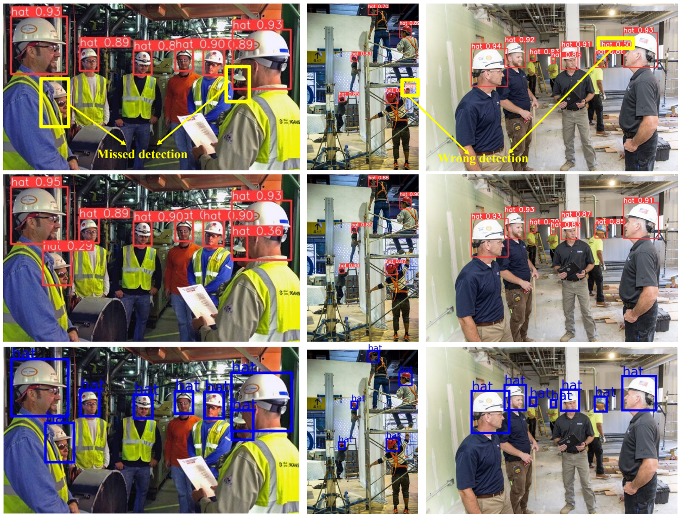
Fig. 9. Visual comparison of inference results between baseline and Mamba-YOLO. The first line represents the baseline inference results, the second line represents the Mamba-YOLO inference results, and the third line represents the manually labeled labels.
