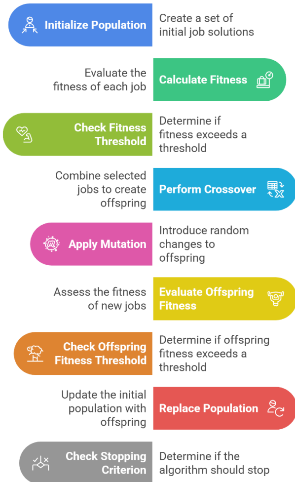
Fig. 3 Process flow diagram of a Genetic Algorithm
