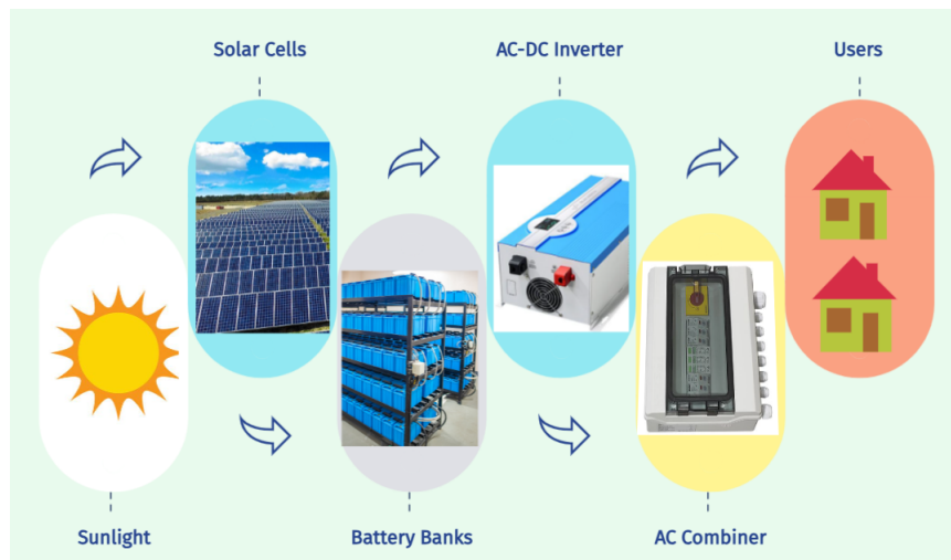
Fig. 1: Solar Power Generation System
