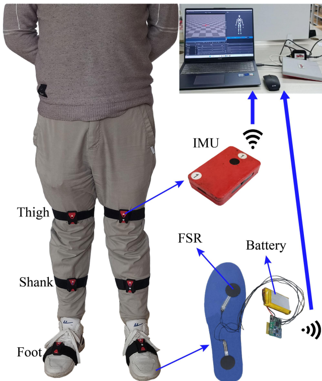
Fig. 1. Data acquisition system with six IMUs on the lower limb and four FSRs inside the shoe.
