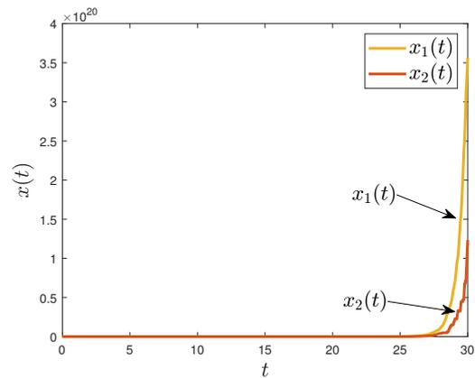
Fig. 1. State trajectories  $x(t)$  without controller  $u(t)$ .
