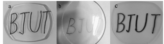
Fig. 17 Comparison of different lenses (a) Polished sample (b) unpolished high-transparency resin sample (c) conventional commercial lens sample
