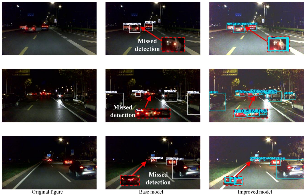
Fig. 13 Comparison diagram of object detection results in real vehicle experiments
