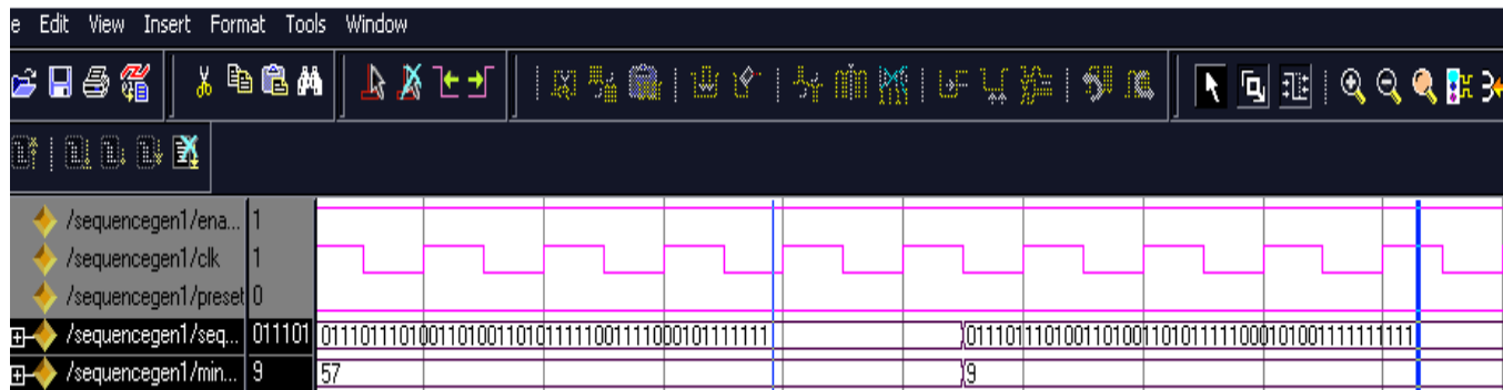
Figure 4: Behavioral simulation result of a good 23-bit Ternary Pulse compression sequence.
