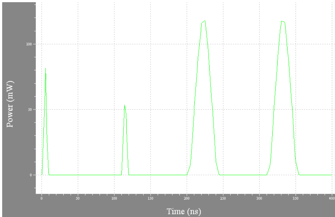
Figure 4. Power waveform for an 8 bit chip inverting the 8 bit video and 16 bit audio data
