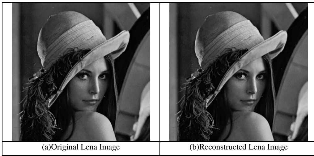
Fig. 3 An example compression result of the Lena image. (a) The 512×512 original gray-level Lena image, and (b) the reconstructed image with a compression ratio 6.847:1 by the modified JPEG-LS codec.
