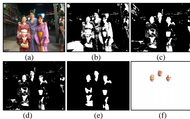
(a) Original image (b) Nonlinear thresholding in RGB color space (c) CBH model thresholding (d) Corrected CBH thresholding (e) Filtering and open/close operation (f) Detected face region
