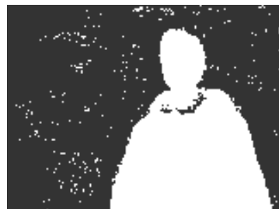
Fig. 3. Result of background subtraction on 'waving trees' using proposed two-layer codebook model
