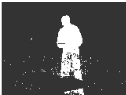
Fig. 6. Result of background subtraction on 'time of day' using proposed two-layer codebook model
