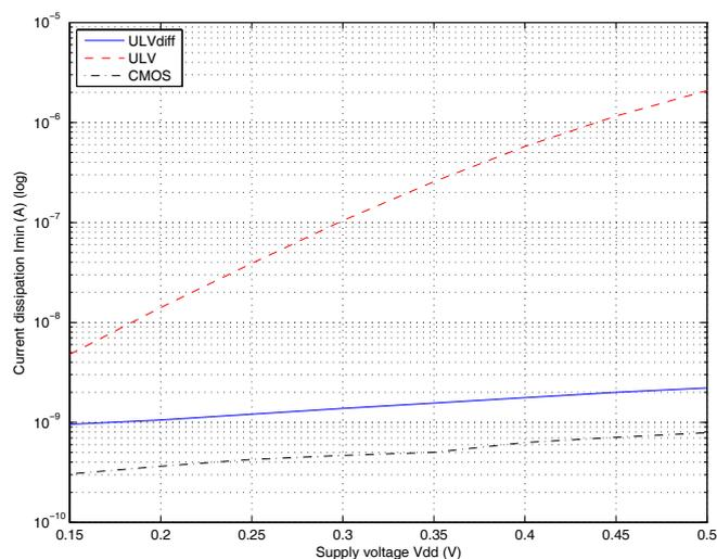
Figure 10: The minimum current dissipation (static dissipation) for all three logic styles.
