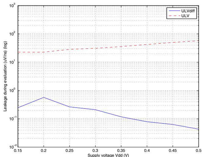
Figure 8: The leakage of the semi floating-gate affecting the output during the evaluation period.
