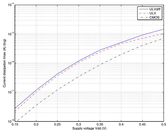
Figure 9: The maximum current dissipation (dynamic dissipation) for all three styles.
