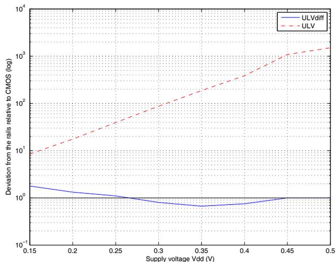
Figure 7: Simulation results showing the deviation for the ULV diff and the ULV relative to CMOS.
