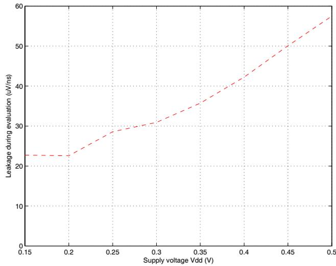
Figure 2: Simulation results show the leakage of the ULV gate during an evaluation period as a function of low supply-voltages. The leakage is given by  $\mu V/ns$ .
