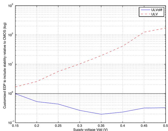
Figure 12: Simulation results for the EDP\*stability for ULV diff and ULV relative to CMOS. The results show an optimum point at  $V_{dd} = 350$  mV.
