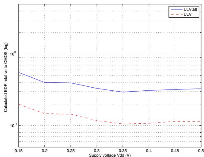
Figure 11: Simulation results for the EDP for the ULV diff and the ULV relative to CMOS.
