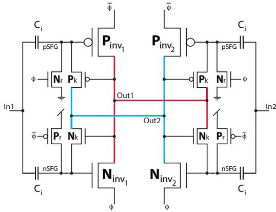
Figure 5: *The ultra low voltage differential semi floating-gate inverter including a keeper function is illustrated. Transistor sizes are kept minimum and matched, the input capacitances are scaled relative to obtain the same voltage attenuation for both nSFG and pSFG.*
