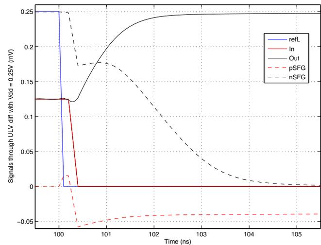
Figure 6: *Simulation results showing all signals in the differential ULV gate during evaluation. As seen from the results the keeper functions steps in at approximately 101 ns and pulling the nSFG down to Gnd.*
