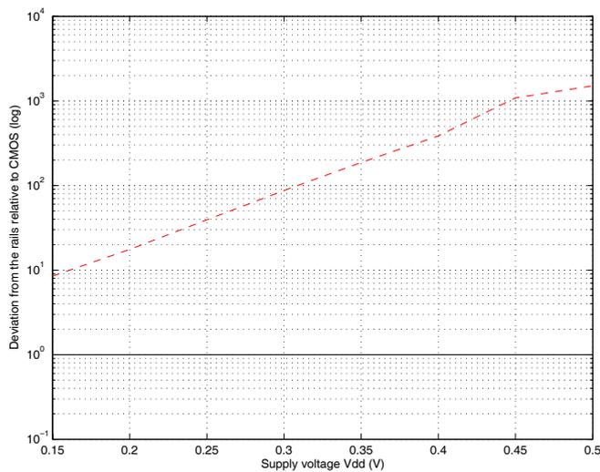
Figure 3: Simulation results demonstrating the amount of deviation relative to CMOS under given supply-voltages. This behaviour is expected due to the leakage through the diffusion contact of the recharge transistor.
