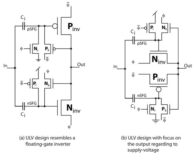
Figure 4: The ultra low voltage gate is modified by including a transistor which acts as an keeper. The keeper transistors are label  $N_k$  and  $P_k$  and would contribute to hold the semi-floating-gates potential, thus eliminating the leakage.
