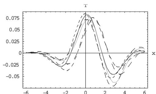
Fig. 3, Comparison for temperature distribution for C-D, G-L and L-S theories, due to moving heat source, times,  $t=0.2$  and  $t=0.5$ .
