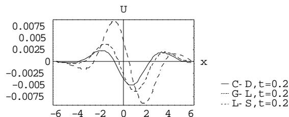
Fig. 13, Horizontal displacement for C-D, G-L and L-S theories, due to moving load at  $t=0.2$
