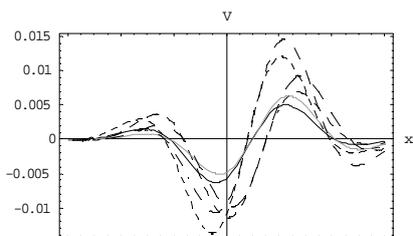
Fig. 9, Comparison for vertical displacement for C-D, G-L and L-S theories, due to moving heat source, times,  $t=0.2$  and  $t=0.5$ .
