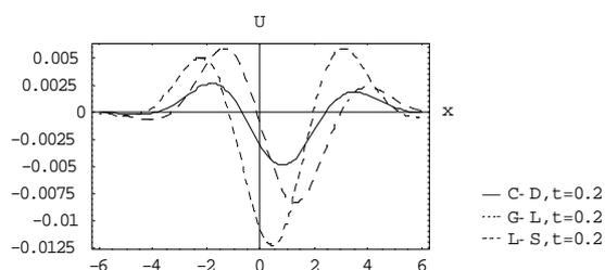
Fig. 4, Horizontal displacement for C-D, G-L and L-S theories, due to moving heat source, at  $t=0.2$
