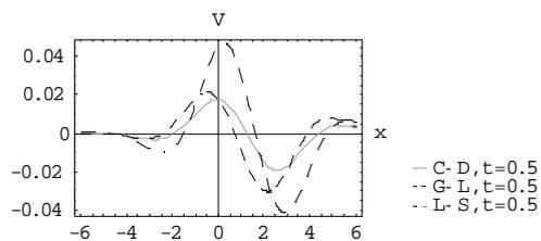
Fig. 17, Vertical displacement for C-D, G-L and L-S theories, due to moving load, at  $t=0.5$
