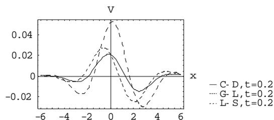
Fig. 16, Vertical displacement for C-D, G-L and L-S theories, due to moving load at  $t=0.2$
