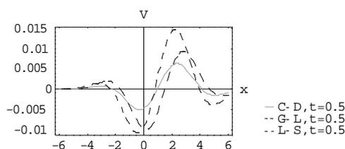
Fig. 8, Vertical displacement for C-D, G-L and L-S theories, due to moving heat source, at  $t=0.5$
