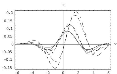
Fig. 12, Comparison for temperature distribution for C-D, G-L and L-S theories, due to moving heat source, times,  $t=0.2$
