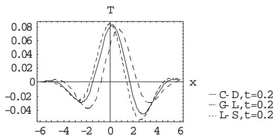
Fig. 1, Temperature distribution for C-D, G-L and L-S theories, due to moving heat source, at  $t=0.2$
