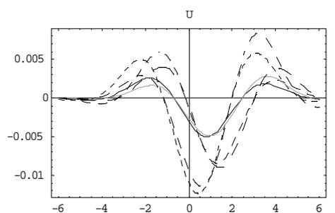
Fig. 6, Comparison for horizontal displacement for C-D, G-L and L-S theories, due to moving heat source, times,  $t=0.2$  and  $t=0.5$ .
