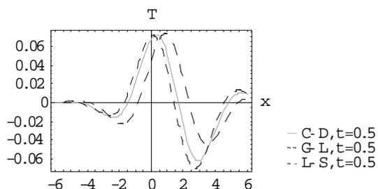
Fig. 2, Temperature distribution for C-D, G-L and L-S theories, due to moving heat source, at  $t=0.5$
