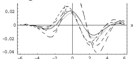
Fig. 18, Comparison for vertical displacement for C-D, G-L and L-S theories, due to moving load at times,  $t=0.2$  and  $t=0.5$ .
