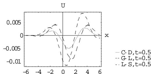
Fig. 5, Horizontal displacement for C-D, G-L and L-S theories, due to moving heat source, at  $t=0.5$
