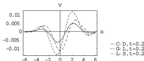
Fig. 7, Vertical displacement for C-D, G-L and L-S theories, due to moving heat source, at  $t=0.2$
