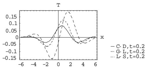
Fig. 10, Temperature distribution for C-D, G-L and L-S theories, due to moving load at  $t=0.2$
