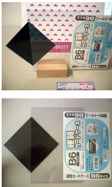
Fig. 10 Quasi-1/2 wave plate (card case)
