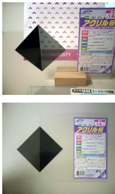
Fig. 9 Quasi-1/2 wave plate (acrylic resin plate)
