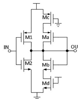
Figure 4. The schematic of the LS circuit
