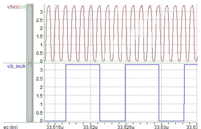
Figure.11 The waveforms of input and output ( $F_{input}=120MHz$ )
