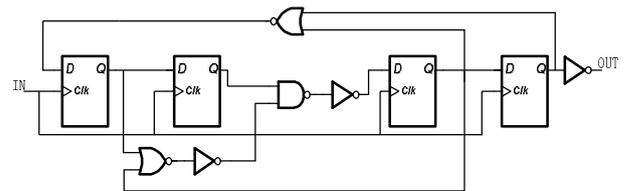
Figure 9. The schematic of divider (N=7)
