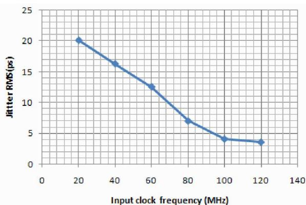
Figure 13. RMS Jitter vs. input frequency
