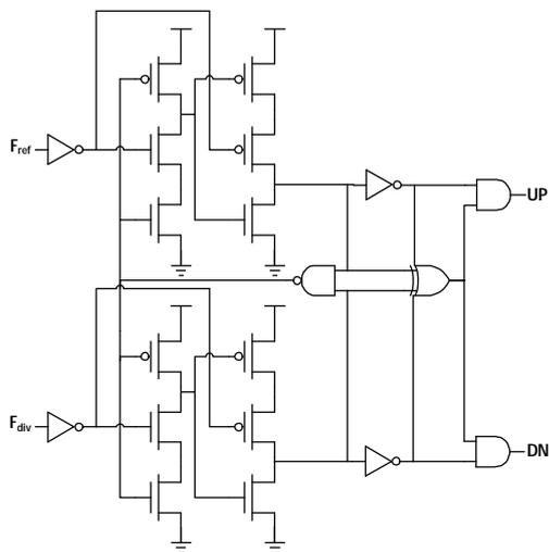
Figure 8. Circuit schematic of the PFD
