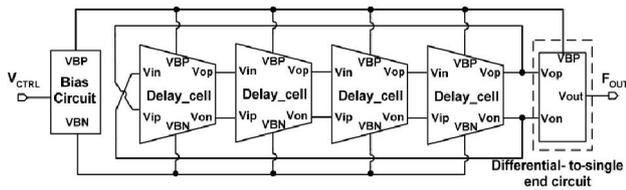
Figure 5. The full VCO circuit
