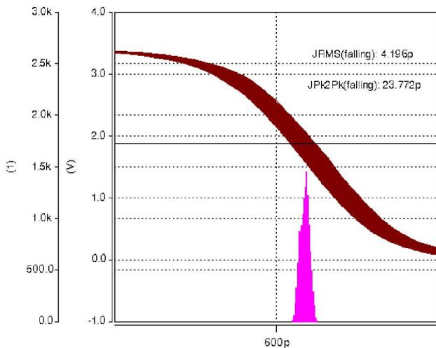
Figure 12. PLL output jitter characteristics ( $F_{input}=120MHz$ )
