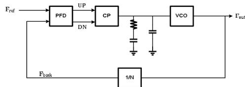
Figure 2. The block of charge-pump PLL
