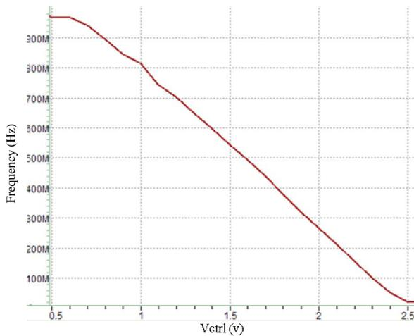
Figure 7. The Tuning curve of the VCO
