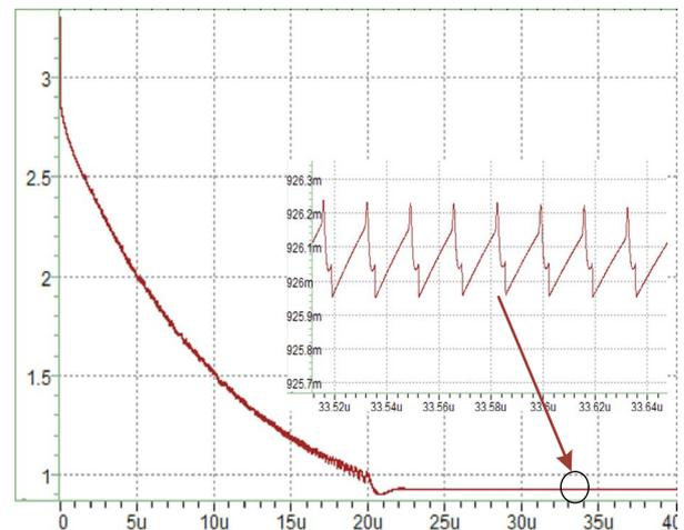
Figure 10 The curves of control voltage ( $F_{input}=120MHz$ )
