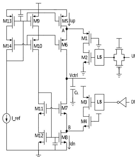
Figure 3. The schematic of proposed charge pump
