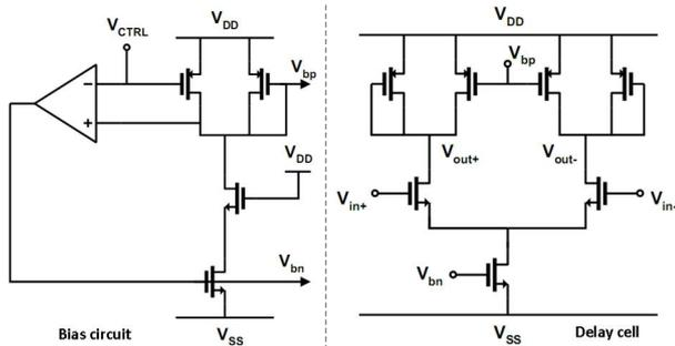
Figure 6. the schematic of Bias circuit and Delay cell
