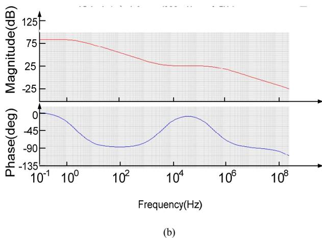
Fig. 7. Simulated frequency response of  $T_c$  in (a) Simulink model and (b) Verilog-A model
