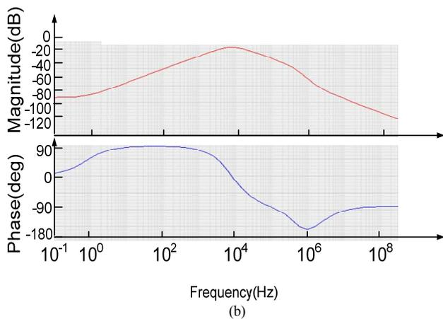
Fig. 8. Simulated frequency response of audio-susceptibility  $G_{vg\_closed}$  in (a) Simulink model and (b) Verilog-A model
