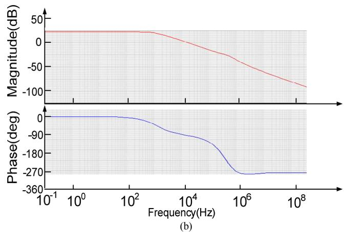
Fig. 6. Simulated frequency response of  $T_a$  in (a) Simulink model and (b) Verilog-A model
