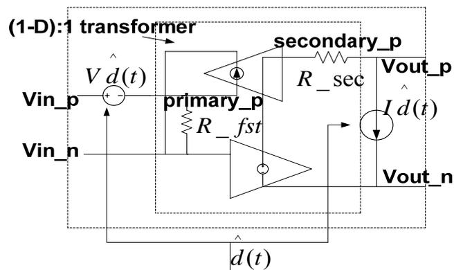
Fig. 2. Insight of packaged power stage linearization part
