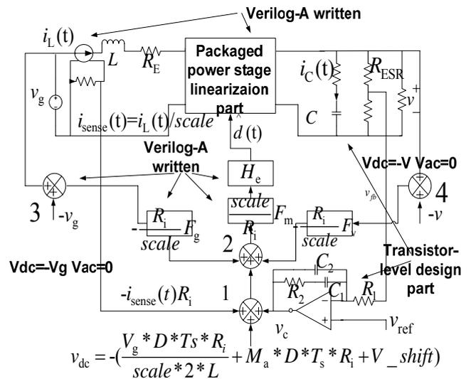
Fig. 1. Continuous-time model based on Verilog-A
