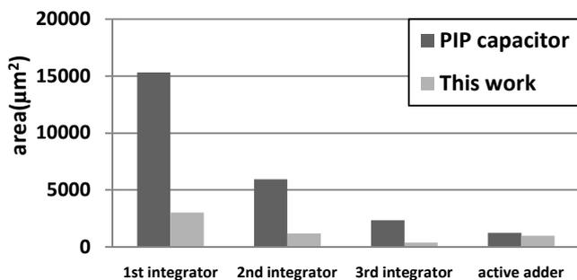
Fig. 9. PIP capacitor area versus MOSCAP area
