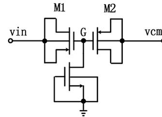
Fig. 5. The MOSCAP in series connection
