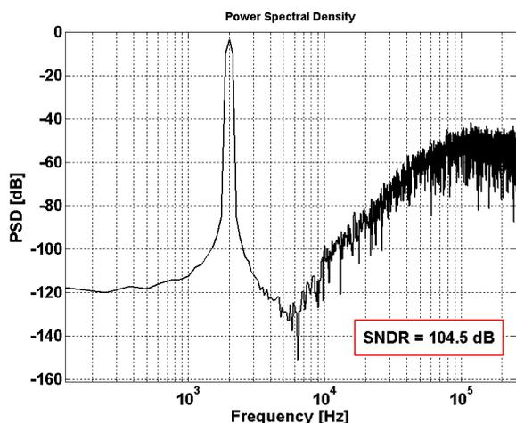
Fig. 10. The simulation results for  $f_{\text{clk}}=512\text{KHz}$ ,  $f_{\text{in}}=2\text{KHz}$  and  $V_{\text{in}}=-1.9\text{dB}$
