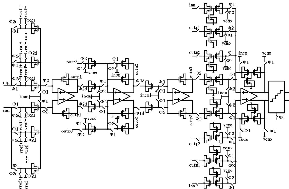
Fig. 8. Modulator circuits with the MOSCAP application
