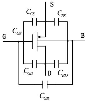
Fig. 2. A P MOSFET and its parasitic capacitance
