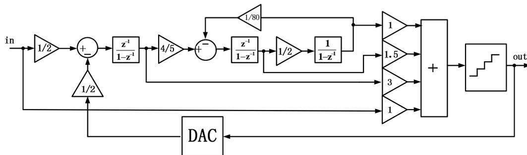
Fig. 7. Behavior model of the Delta-Sigma modulator
