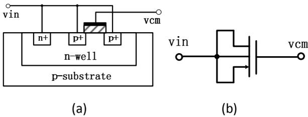
Fig. 3. (a) The crossover section and (b) the circuit of a PMOSFET MOSCAP
