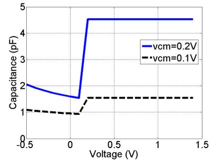
Fig. 6. C/V feature of series compensated MOSCAP
