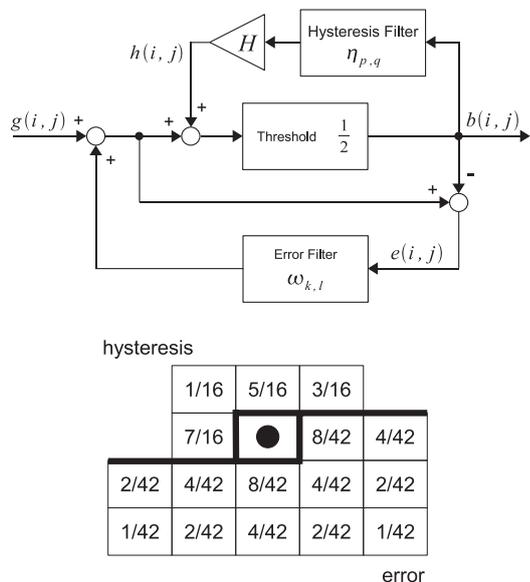
Figure 3: The block diagram of the EDODF and its error filter
