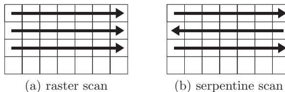
Figure 5: Two commonly used scanning path for the Error Diffusion
