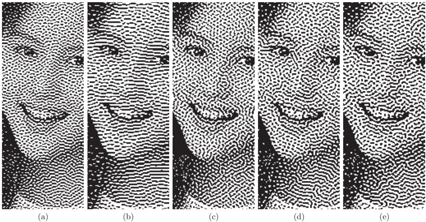
Figure 11: The resulting binary images for a woman image, (a) EDODF ( $H = 0.5$ ), (b) EDODF ( $H = 0.75$ ), (c) Cluster-dot error filter, (d) Cluster-dot error filter with feedback ( $H = 0.1$ ), and (e) Cluster-dot error filter with feedback ( $H = 0.15$ )
