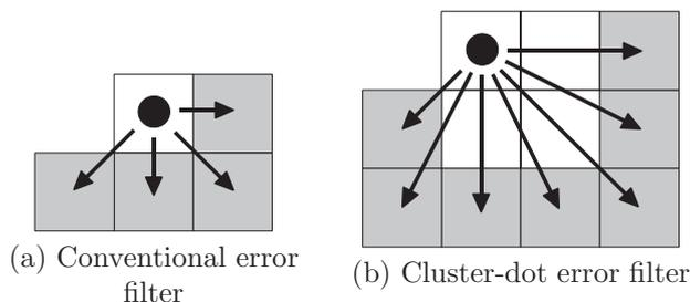
Figure 4: Conventional and cluster-dot error filters
