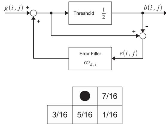
Figure 2: The block diagram of the Error Diffusion and its error filter
