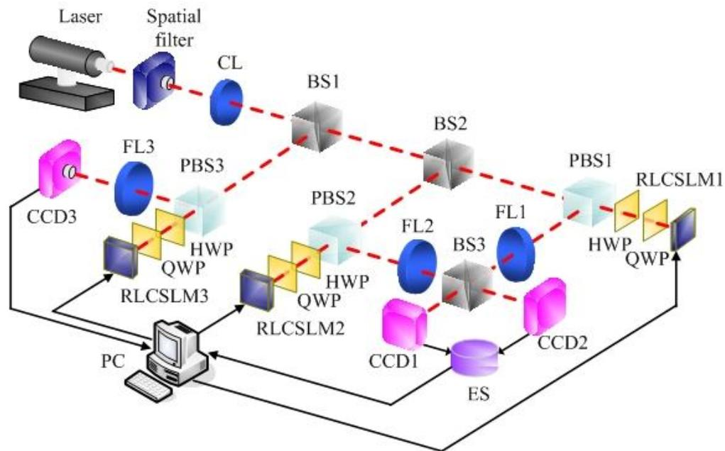
Figure 1. The structure of a MZJTC system.
