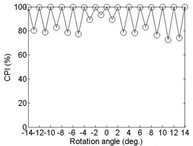
Figure 5. CPI versus rotation angle from  $-14^{\circ}$  to  $14^{\circ}$ .
