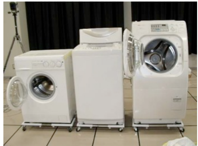
Figure 1. Laundry machines: European washer AWD-500, vertical-drum washer ASW-800, and slanted-drum washer-dryer AQ-1 (left to right).
