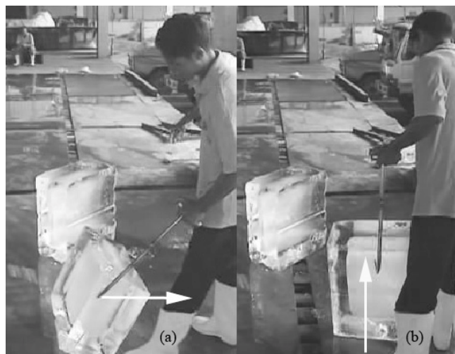
Fig. 1. Illustration of turning side up process starting with (a) Pulling, and then (b) lifting
