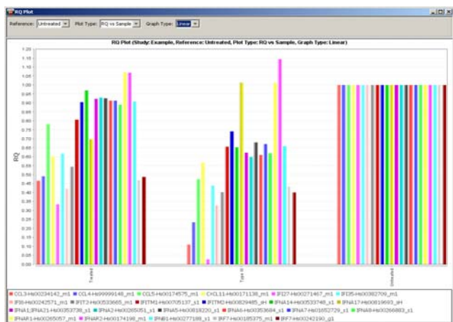
Fig. 7 RQ Plot. It shows the RQ (fold change) versus Target (gene) or RQ versus Sample, as Linear, \log_{10} , or \log_2 scale. The standard deviation is also displayed as error bar for each sample on \log_2 scale when no biological group is specified.
