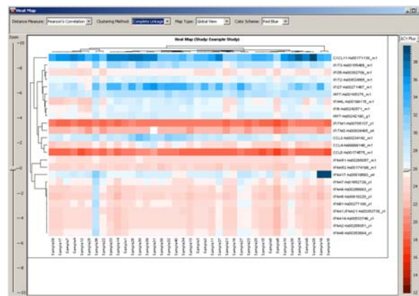
Fig. 8 Dendrogram and Heat Map. It displays the dendrograms of both sample cluster and gene cluster along with gene expression heat map. Genes and samples are clustered using hierarchical clustering [5] with average linkage, complete linkage or single linkage method. The normalized gene expression data ( \Delta C_T ) are used to calculate the distances between samples and genes using either Pearson's correlation coefficient or Euclidean distance. The heat map can be configured as either red-blue or red-green map, with red color box representing up-regulated gene expression level, and the middle expression level can be set using the adjustable color scale on the right side.
