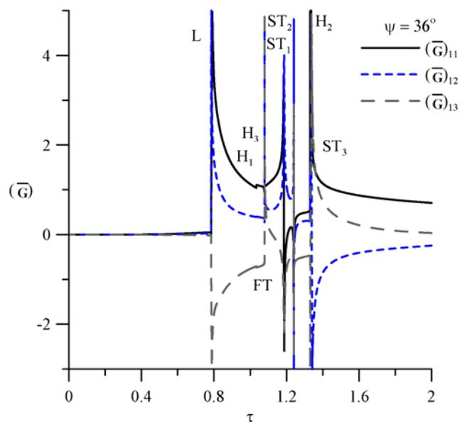
Figure 3. The components of Green's functions  $(\bar{G})_{11}$ ,  $(\bar{G})_{12}$ , and  $(\bar{G})_{13}$  for  $\psi = 36^\circ$ .
