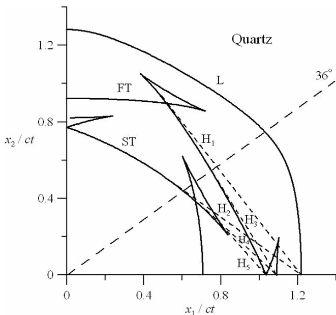
Figure 1. Wavefronts and the angle of observation for quartz.
