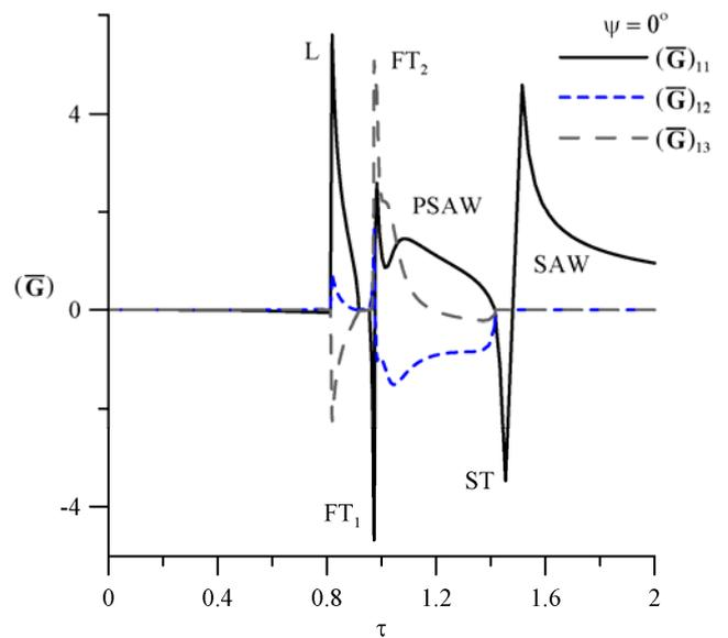
Figure 2. The components of Green's functions  $(\bar{G})_{11}$ ,  $(\bar{G})_{12}$ , and  $(\bar{G})_{13}$  for  $\psi = 0^\circ$ .
