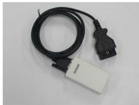
Fig. 6. EZ-SCAN5 OBD-II to Bluetooth adapter.
