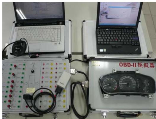
Fig. 11. The simulation equipments of the proposed speech-controlled real-time remote vehicle OBD system.
