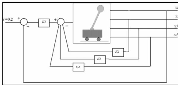
Fig. (1): Block diagram of SIP and state feedback controller.
