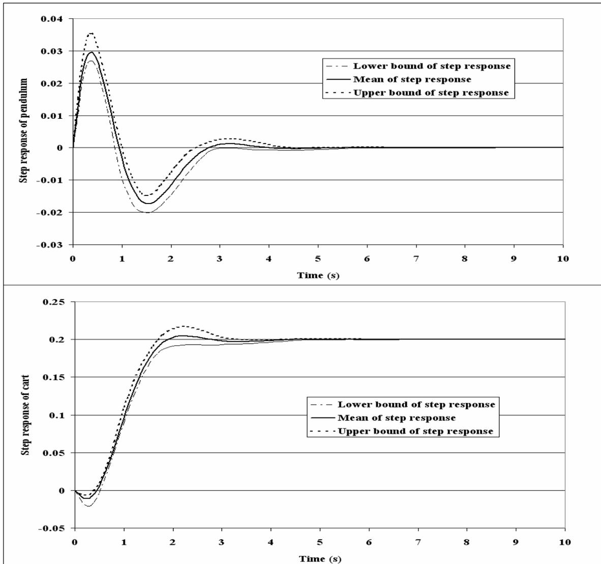
Fig. (3): Probabilistic time response behaviors of optimum design point M (7000 samples).
