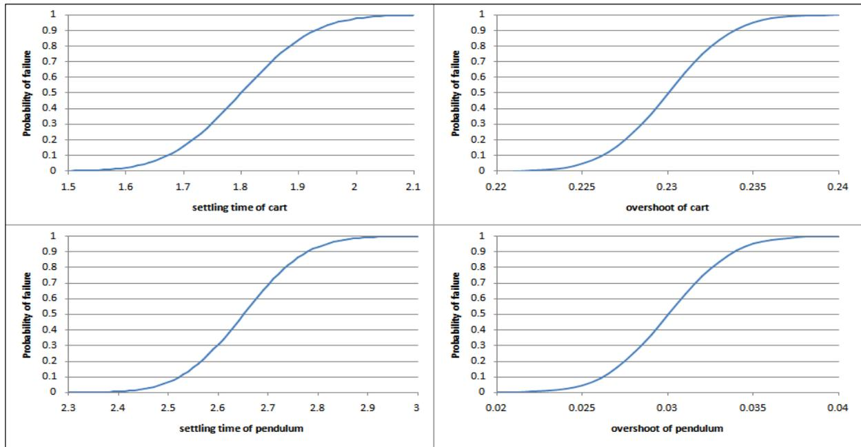
Fig. (2): fuzzy threshold values for calculating the probability of failure
