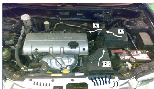
Fig. 3 AIS located under the bonnet of Waja 1.6
