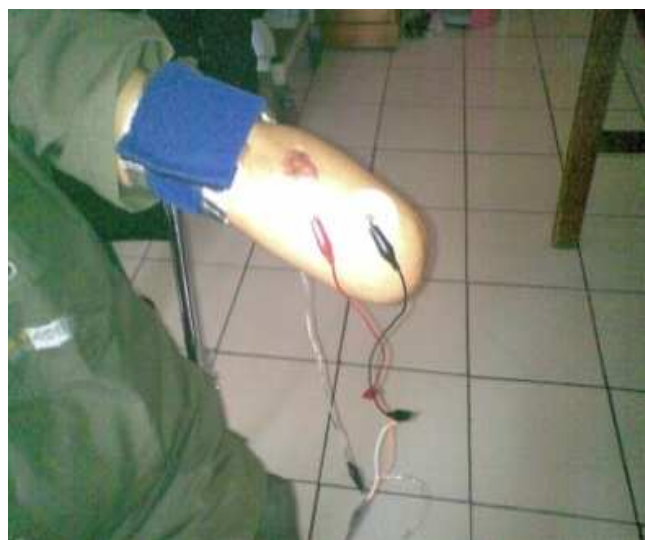
Fig. 3. Allocate neutral probe and electrodes of MES catcher in amputee.
