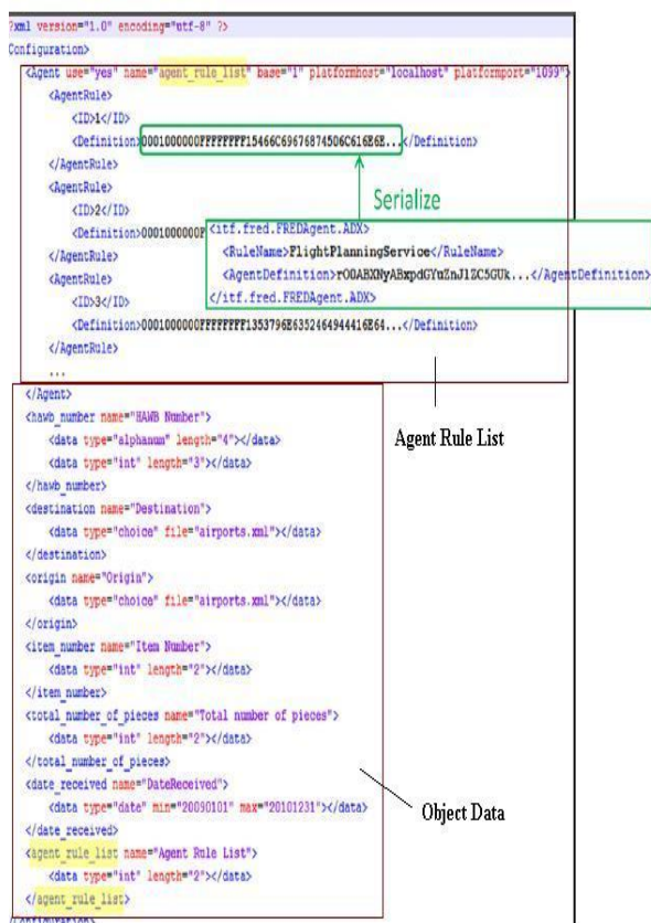
Fig. 2. Example of the A-FRED schema
