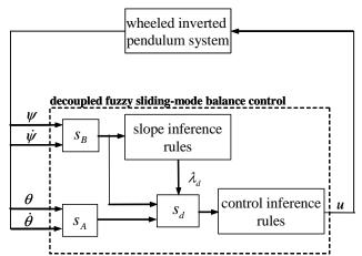
Fig. 3. The black diagram of the proposed DFSBC system.
