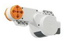
Fig. 2. The used 9V DC servomotor.
