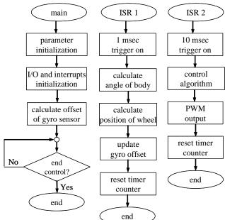
Fig. 6. The software flowchart.
