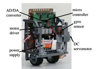
Fig. 5. The experimental setup.
