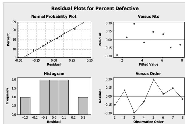
Fig. 7. Residual plots for percent defective ( $2^{k-1}$  design)
