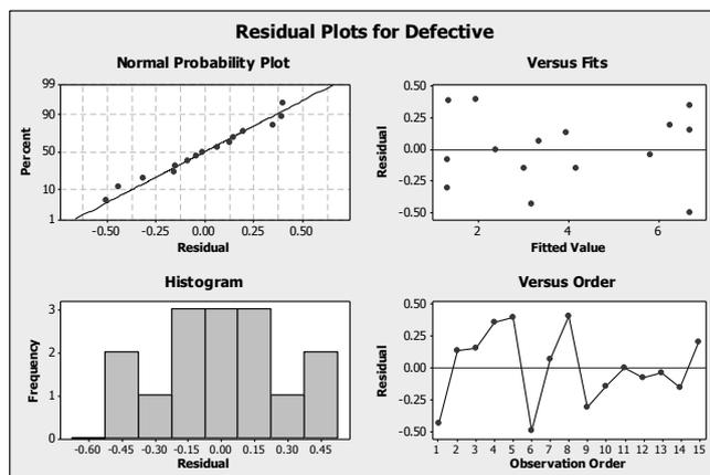
Fig. 9. Residual plots for percent defective (Box-Behnken)
