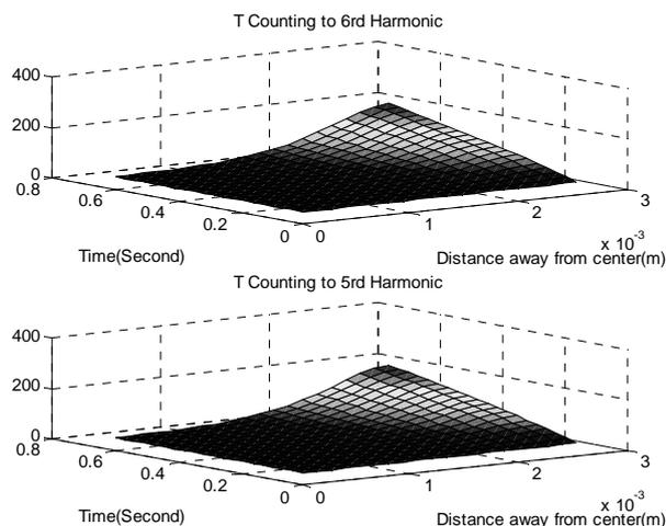
Fig. 4 Temperature rises caused by the first 6 and the first 5 components make no obvious difference.
