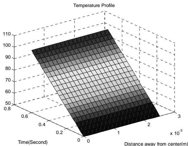
Fig. 5 Temperature rises caused by the very low frequency excitation. The current distributes evenly on cross section and finally lead to uniform temperature profile at each constant.
