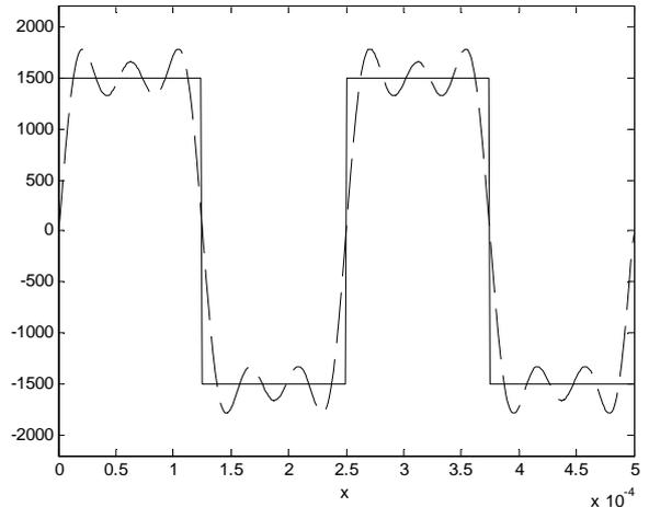
Fig. 3 Square wave (solid line) and Fourier expansions sum (dashed line) counting up to 5rd harmonic. The appropriate number of decomposition to be taken depends on the influence on temperature rise on hottest spot of high order harmonics.
