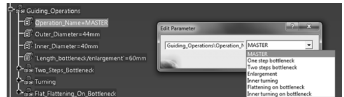
Fig. 4. CATIA software screenshot showing the parameters from „Guiding operations“ group
