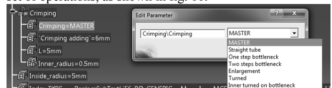
Fig. 10. CATIA software print screen showing the parameters of Crimping
