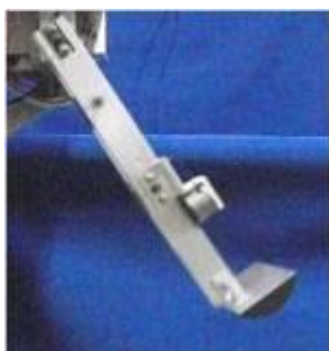
Fig. 10. Leg in the case that rebound of the knee is suppressed by the magnetic force
