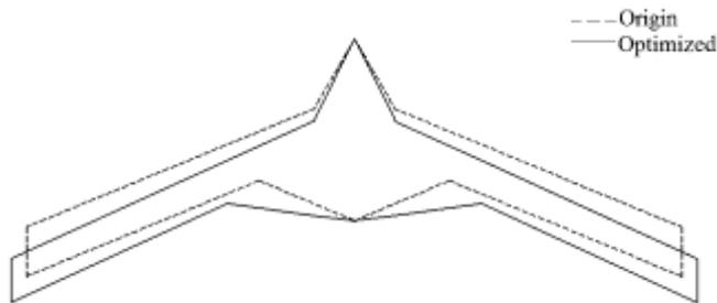
Fig. 10. Comparison of the aircraft outline between initial and optimized.
