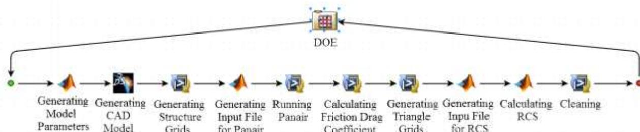
Fig. 5. DOE Flowchart of UAV.
