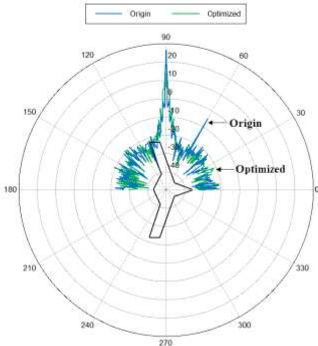
Fig. 14. Distribution comparison of UAV RCS.
