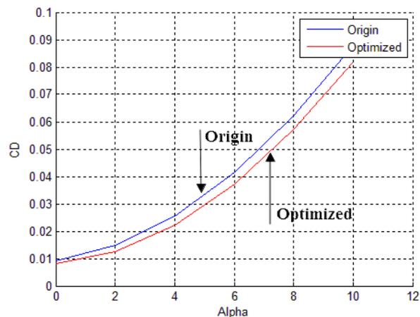
Fig. 12. Drag coefficient comparison of UAV.
