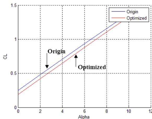
Fig. 13. Lift coefficient comparison of UAV.
