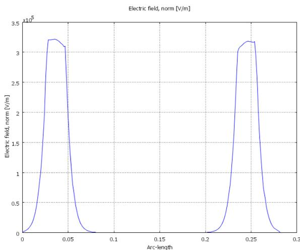
Fig. 15 Electric field and potential Distributions along reference line 3 on hydrophilic and polluted surface insulator condition with lower-upper air gaps.
