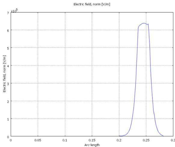
Fig. 13 Electric field and potential Distributions along reference line 4 on hydrophilic and polluted surface insulator condition with lower air gap.
