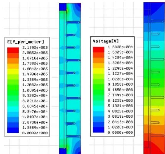
Fig. 4 Electric field and potential Distributions along reference lines on clean and dry insulator condition
