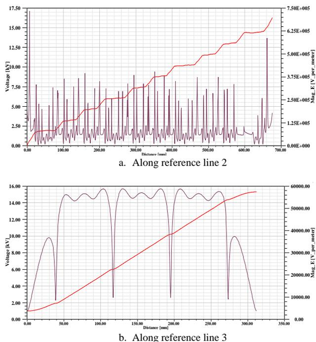
Fig. 6 Electric field and potential Distributions along reference lines on hydrophobic and polluted surface insulator condition with lower air gap.
