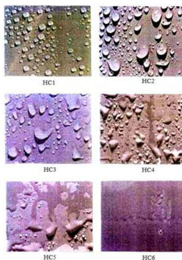
Fig. 1 Hydrophobicity Classification Guide
