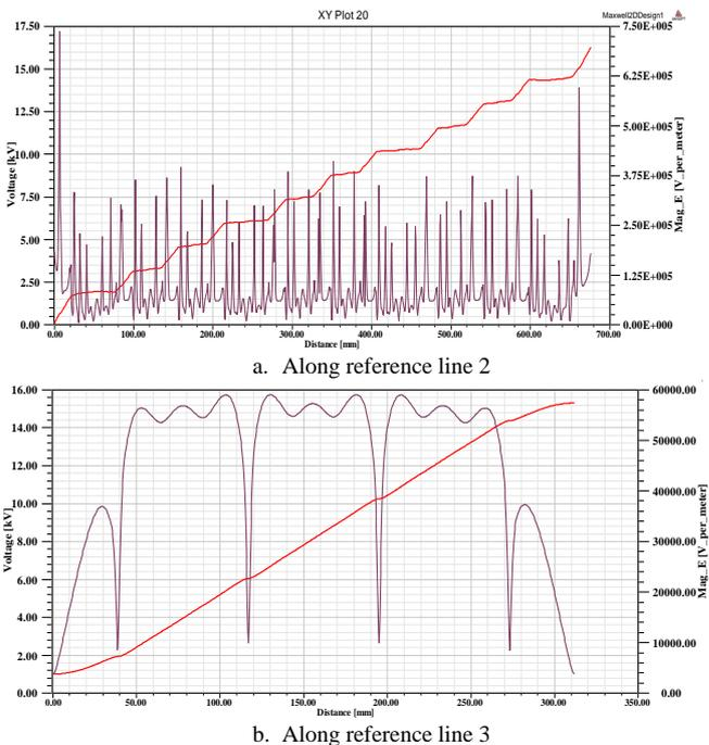
Fig. 5 Electric field and potential Distributions along reference lines on hydrophobic and polluted surface insulator condition, and without air gap.
