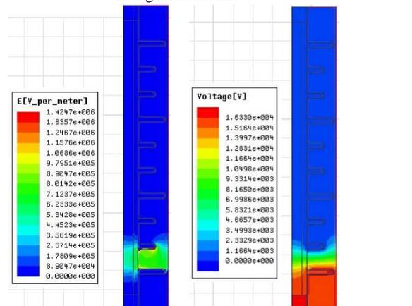
Fig. 10 Electric field and potential Distributions along reference lines on hydrophilic and polluted surface insulator condition with lower air gap.
