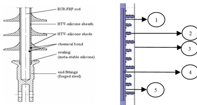
Fig. 2 Structure of composite insulator with reference lines and dry bands location
