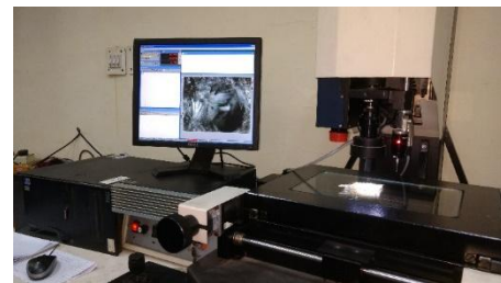
Fig. 2: Calculating F_d on the Vision Inspection System
