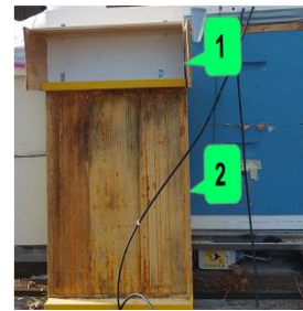
(a) Protection box from inside (1); box is attached to a hive lid with screws and metallic brackets (2).
