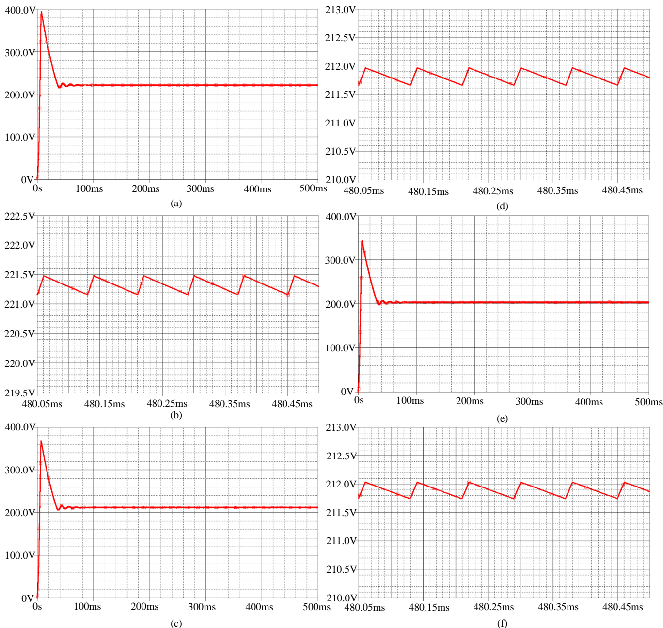
Fig. 4. Steady-state responses of MSCCI. (a) V_O for V_{ref}=220V , (b) rp=0.144\% , (c) V_O for V_{ref}=210V , (d) rp=0.143\% , (e) V_O for V_{ref}=200V (f) rp=0.141\% .
