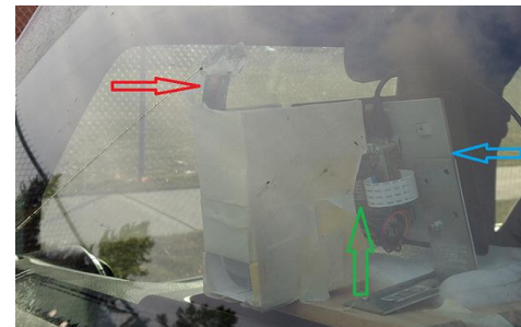
Fig. 4. An RPi camera board v2 (red arrow) attached to small cardboard box for balance and taped to windshield; RPi computer (green arrow); RPi monitor (blue arrow).
