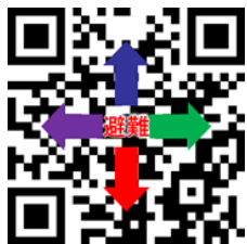
Fig. 1. A QR code with arrows. The arrows are used to indicate a path recommended by the evacuation support system.
