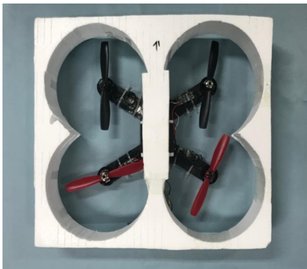
Fig. 1. Top view of the developed drone system installed with guard plate for adhering function
