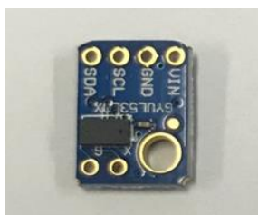
Fig. 5. Distance sensor (VL53L0X, ST Microelectronics Co., size: 13.3mm * 10.5mm * 2.4mm, weight: 0.5g)
