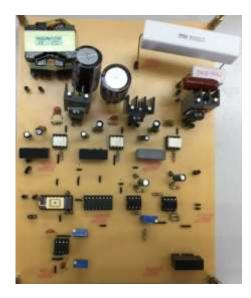
Fig. 6. Prototype circuit of closed-loop SCII.
