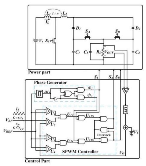
Fig. 1. Configuration of closed-loop SCII.
