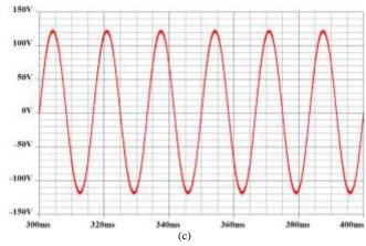
Fig. 4. Output  $V_{OUT}$  for  $V_{REF}$ : (a)  $f_O$  =60Hz,  $V_m$  =145V; (b)  $f_O$ =60Hz,  $V_m$ =135V; (c)  $f_O$  =60Hz,  $V_m$ =125V.
