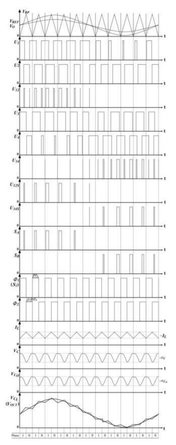
Fig. 2. Theoretical waveforms of closed-loop SCII.
