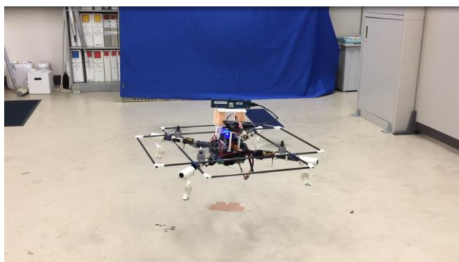
Fig. 10. Hovering motion in experiment of testing automatic flight of the developed system
