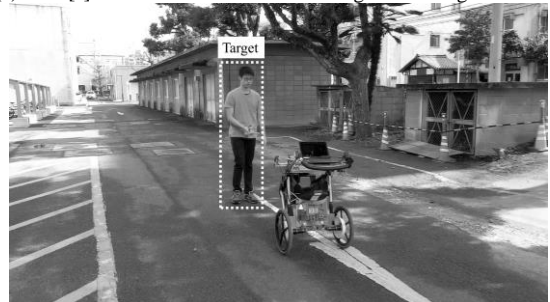
(d) t = 11 [s]: The mobile robot is stopped according to the motion of the target in safety area
